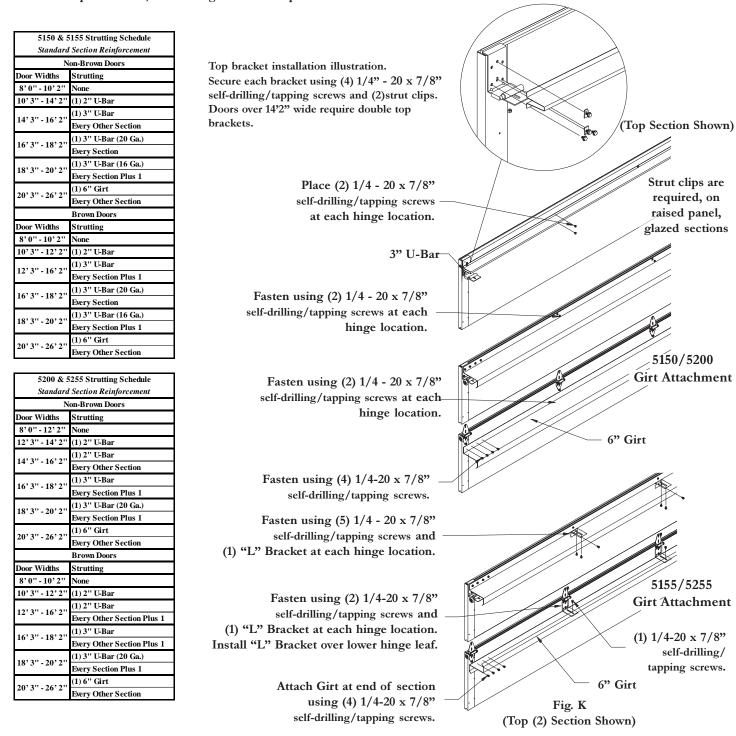
STEP 5. Center and level (or support to a known grade level) the bottom section in the opening, as seen in Fig. K. Temporarily attach the vertical tracks to the jambs. Allow 1/2" clearance between the section and the track as illustrated in the sideroom illustrations (page 3).
